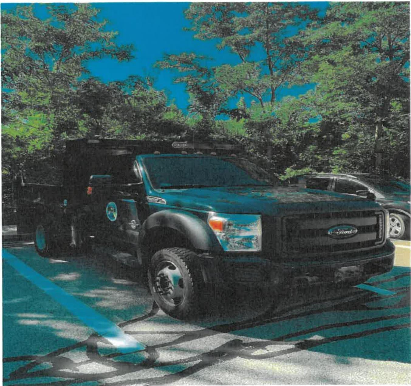
The requested equipment will replace a 2014 Ford F550 6-wheel dump truck with a steel dump body and a slide in salt/sander unit. This truck is equipped with a nine-foot plow and a seven-foot wing blade.
