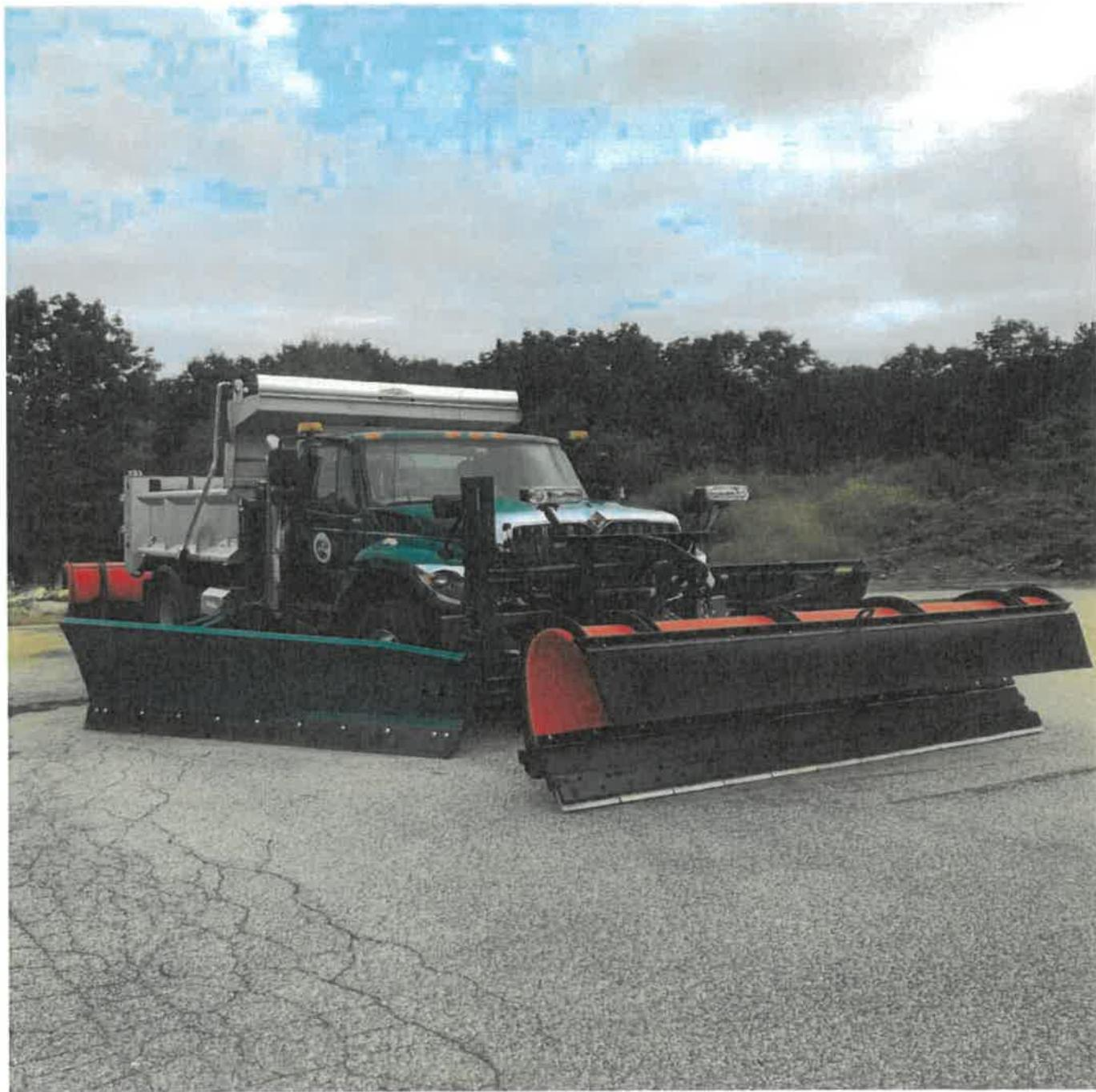
The equipment requested will replace a 2014 International Model 7400 SFA - 6-wheel dump truck with an all-season side dump body with integral conveyor and sander. This truck is equipped with an 11-foot plow and a 10-foot wing blade.
