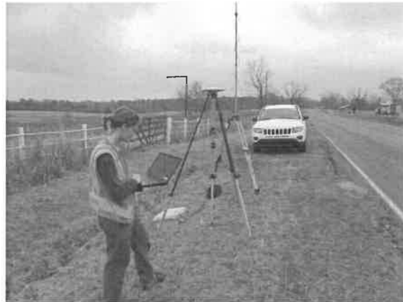
Figure 4. NV5 Geospatial's surveying crews are equipped with state-of-the-art robotic total stations and real time kinematic GPS receivers.
