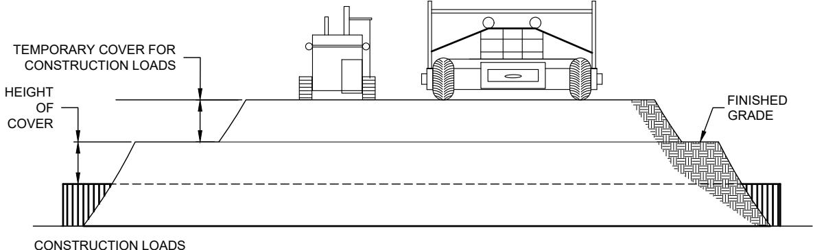
FOR TEMPORARY CONSTRUCTION VEHICLE LOADS, AN EXTRA AMOUNT OF COMPACTED COVER MAY BE REQUIRED OVER THE TOP OF THE PIPE. THE HEIGHT-OF-COVER SHALL MEET THE MINIMUM REQUIREMENTS SHOWN IN THE TABLE BELOW. THE USE OF HEAVY CONSTRUCTION EQUIPMENT NECESSITATES GREATER PROTECTION FOR THE PIPE THAN FINISHED GRADE COVER MINIMUMS FOR NORMAL HIGHWAY TRAFFIC.
