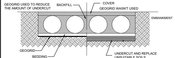
GRADE THE FOUNDATION SUBGRADE TO A UNIFORM OR SLIGHTLY SLOPING GRADE. IF THE SUBGRADE IS CLAY OR RELATIVELY NON-POROUS AND THE CONSTRUCTION SEQUENCE WILL LAST FOR AN EXTENDED PERIOD OF TIME, IT IS BEST TO SLOPE THE GRADE TO ONE END OF THE SYSTEM. THIS WILL ALLOW EXCESS WATER TO DRAIN QUICKLY, PREVENTING SATURATION OF THE SUBGRADE.
