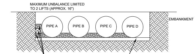
IF AASHTO T99 PROCEDURES ARE DETERMINED INFEASIBLE BY THE GEOTECHNICAL ENGINEER OF RECORD, COMPACTION IS CONSIDERED ADEQUATE WHEN NO FURTHER YIELDING OF THE MATERIAL IS OBSERVED UNDER THE COMPACTOR, OR UNDER FOOT, AND THE GEOTECHNICAL ENGINEER OF RECORD (OR REPRESENTATIVE THEREOF) IS SATISFIED WITH THE LEVEL OF COMPACTION.
