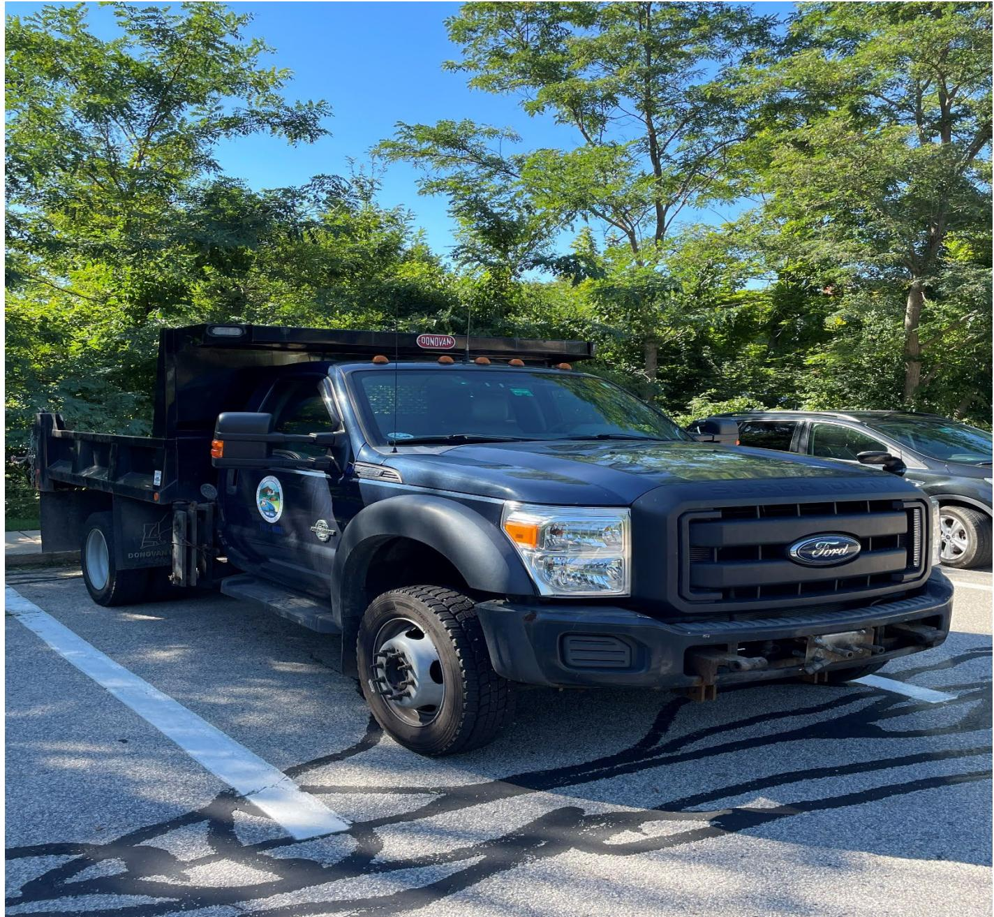
The requested equipment will replace a 2014 Ford F550 6-wheel dump truck with a steel dump body and a slide in salt/sander unit. This truck is equipped with a nine-foot plow and a seven-foot wing blade.
